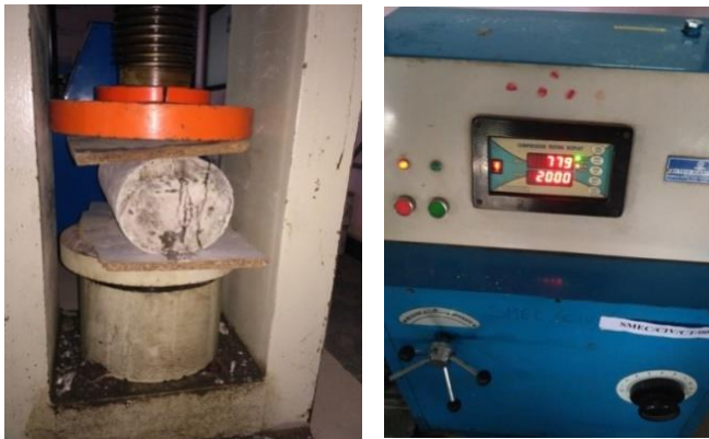
Fig-3: Testing of cylinders
